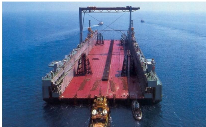
FIGURE 2 FLOATING DRY DOCK [1]
